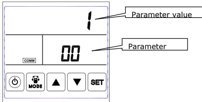
After entering the parameter setting interface, press SET button shortly to change the parameter number, every pressing will make parameter value +1. After choosing the correct parameter number, press Mode button for short, parameter value flashes at the top right corner, at this time to change the value by UP and DOWN buttons. After parameters setting then press SET button to save.
